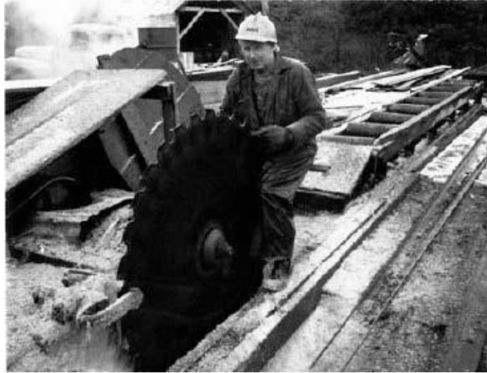
Albert Lee, long-time employee at the logging camp, sharpening the 54-inch circular saw in the sawmill where Eileen and I cut all the cedar and spruce lumber for our cabin in Winter Harbour. Photo: Bill Moore
